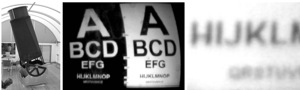
Figure 16. Reflections in a tea pot, taken from a large distance of 30 meters using a larger telescope. The 18pt font is readable from the reflections.
