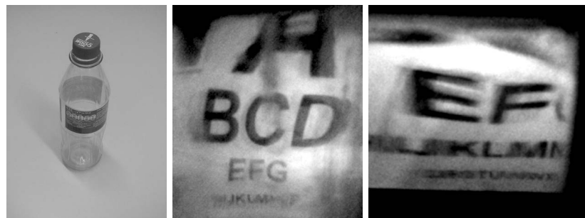
Figure 12. Reflections in a 0.5l plastic Coca-Cola bottle, taken from a distance of 5m. Because of the irregular surface, only parts of the text are readable.
