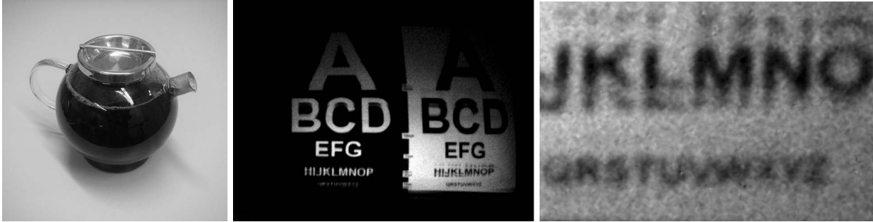
Figure 5. Reflections in a tea pot, taken from a distance of 10m. The 18pt font is readable from the reflection.
