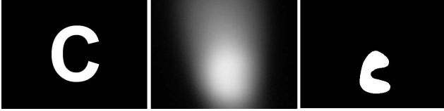
Figure 18. Diffuse reflections of a monitor display from a wall, recovered using deconvolution algorithms: The monitor image (left), the reflection from the wall (middle), and the result from deconvolution, gamma correction, and edge detection (right).
