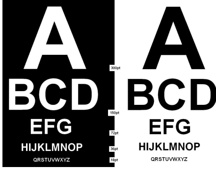
Figure 4. The test image used in most of our experiments. Font sizes are 300pt, 150pt, 72pt, 36pt, and 18pt.
